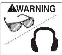
Operating this nailer can propel objects into the air, causing immediate eye damage. To protect yourself, always wear American National Standards Institute (ANSI) approved safety glasses or goggles when operating this equipment. In addition, this nailer discharges at 85-90 decibels. To protect your hearing, always wear ANSI approved ear protection when operating this nailer.
